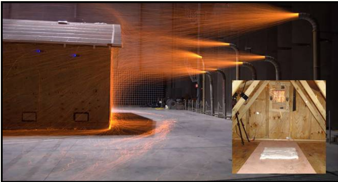
Vulnerability of Vents to Wind-Blown Embers. Credit: IBHS
