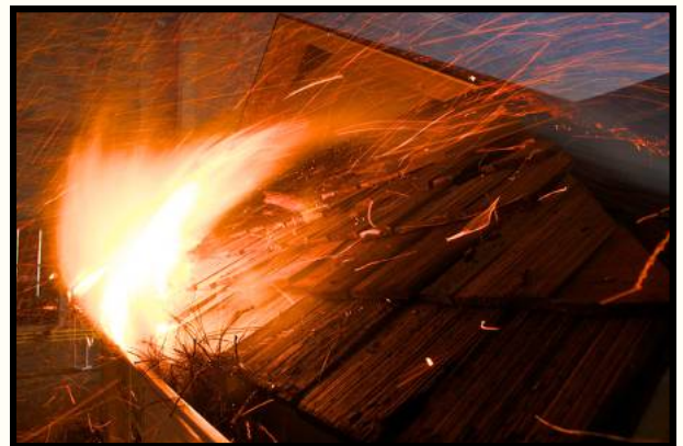
Embers ignite pine needles in gutter during an IBHS home ignition simulation. Credit: National Geographic
